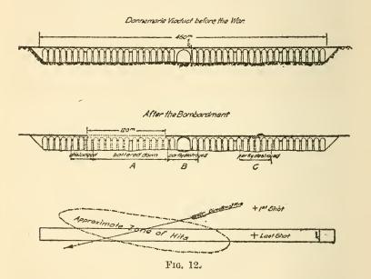
arches were severely damaged. The Germans had waited until the reconstruction was completed and then bombarded it, the fire being directed by aviators.
