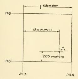
FIG. 4.— OLD FRENCH SYSTEM. Kilometer Square. Coördinates of Point "A" Written as Follows, in Full: 243.75—175.22, or Abbreviated: 375.522.
